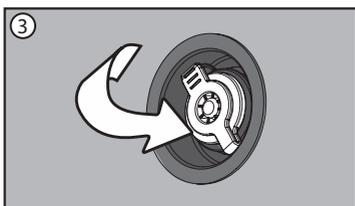
Fully remove pump and close external stopper.
