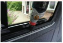
Using a 2.5mm metal drill bit - choose one of the pre-drilled rail holes and drill through the van metal work. A Stanley knife is useful to remove any lining carpet that gets caught round the drill bit.
