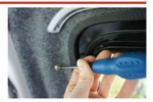
Using the side poppers on each curtain as a location guide, mark and drill the van metal work. Screw the 'male' popper to the van window recess.
