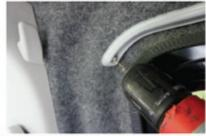
Insert the plastic end stops into the top rail and, using the hole in each as a guide, drill right through the rail and the van metal work.
