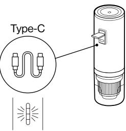
Use type-C cable for charging. When connecting to the cable, the lights will turn on according to the power status. When fully charged, the lights will turn off in 1 minute.
