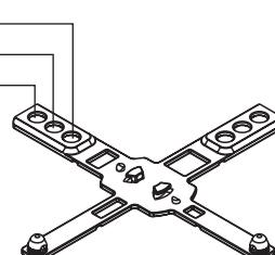
3. Connect the base crosses in the desired position by pressing them down firmly. Please use the assembly tool provided for this purpose. Please never use a hammer or other such tools!
