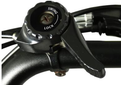
When getting on the bike, the swivel mechanism must be blocked, the lever must be on LOCK as shown in the illustration.
