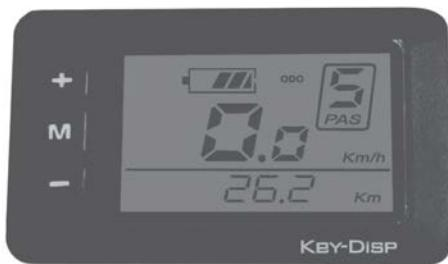
The control unit is integrated with the LC-Display and operates the drive system. It is located on the handlebar.
