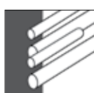
Sharpened pipe ends for the most common pipe diameters
