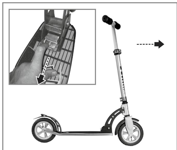
Push forward the steering bar and pull the rail in the direction of the arrow. Now collapse the scooter back.
