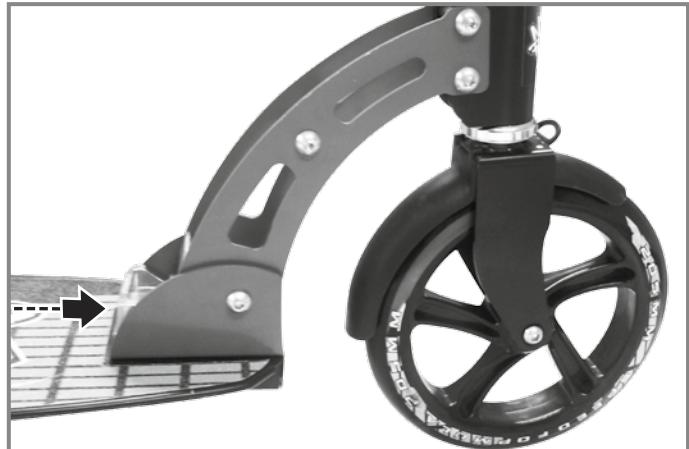
Please ensure before using the scooter that when it is snapped out in place, the rail snaps back correctly automatically.
