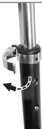
Open the quick-release lever and slide in the handlebar stem by pressing in the click closure.
