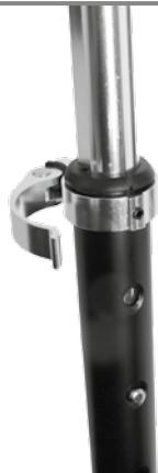
Open the quick-release lock and pull out the handlebar stem until the automatic latch engages. Then close the quick-release lock again. The clamp tension of the quick-release lock can also be adjusted by tightening or loosening the securing nut.
