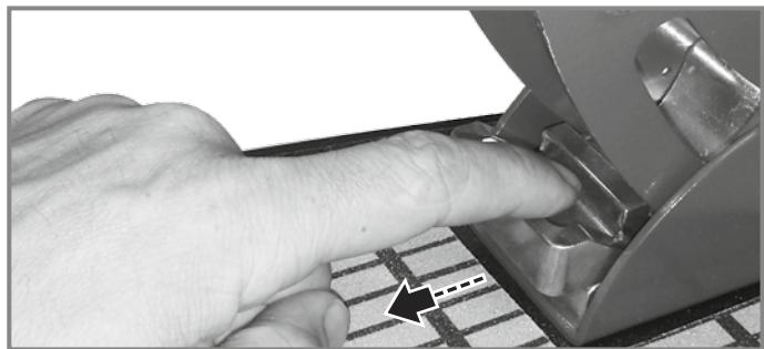
Pull the rail of the snap fastener backwards towards the rear wheel.
